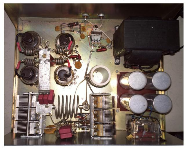
I thought long and hard about putting a filter network on the top of the chassis between the switching relay and the tank coil. A hole and grommet could be put in the deck, and the filter could go in a small metal box. However, voltages run high there, and I was worried about arcing, feedback, etc. I decided that under the deck was best.
