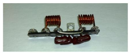
I bought the filter below from a Russian eBay seller, R3KB04. This is a 2-section T-Filter, especially well-suited for low impedances. I was testing it in this picture. Note the cutoff frequency, marked on the filter. This worked so well, it became the "one to beat". My plan is to install this in another small linear that I have that also lacks an input filter.
