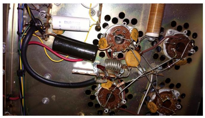
The sites predicted that this filter would roll off before the frequency reached 10 meters, and interestingly, after my 930S tried repeatedly to tune up on 10 meters, the inductor was hot.
