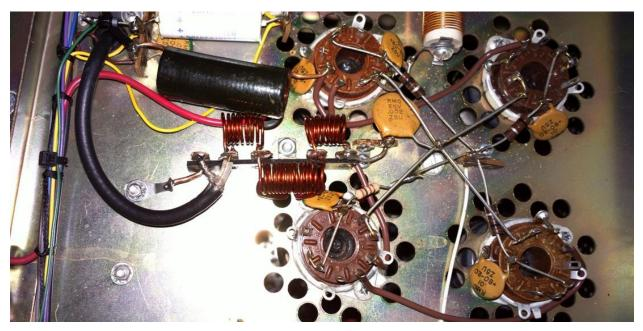
This filter worked very well, allowing my Kenwood tuner to work with all the bands from 10M to 80. The only problem was that the air-core design resulted in significant attenuation of the input signal. I lost at least 50 watts output.
