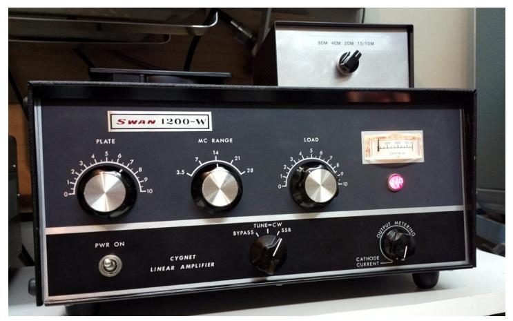
This amp is a prime candidate for mods, because it has lots of room inside. It produced about 400 watts PEP out of the box with the 6JE6's that came in it. Only one tube was "down" a little, and it was a Realistic brand tube.
