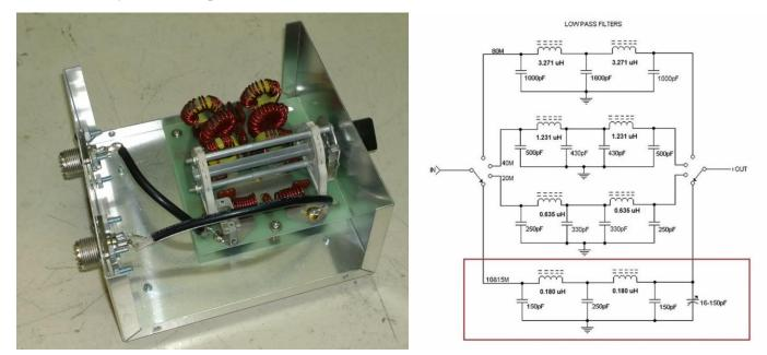
Note that the 10-15M filter portion of the Palomar LPF uses air inductors, and the rest are toroidal. The picture below shows my copy of this filter. I didn't have the correct adjustable trimmer in my parts bin, so I measured the value of the trimmer in the Palomar filter using my LCR and installed a fixed capacitor instead. This worked, but not as well as the one in the Palomar LPF, and it reduced my output. So, I decided to keep looking
