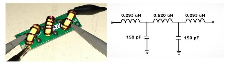
The parts values you see in the schematic aren't marked on the filter. I used my new CEM LCR to find the values. I unsoldered one end of each toroid to accurately read its value. This filter worked great in my 1200-W, but the large diameter coils made it too tall to fit under the deck. I decided to duplicate their filter using air-core coils.
