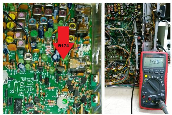
I strongly suggest using a J-clip lead for testing. Be careful not to rock R174 back and forth as you remove the paint or you may loosen it. I would use an Exacto knife and work slowly, shaving in the direction of the wire.
