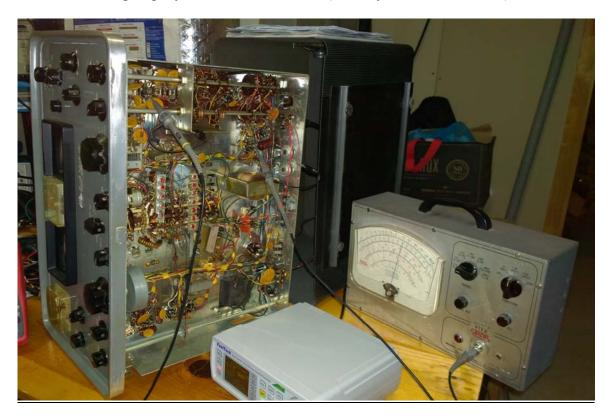
Testing a pair of DMMs for frequency response at 5 & 30 MHz
