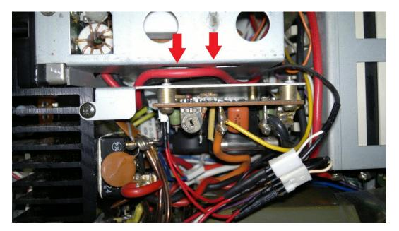
**Inspection.** Carefully examine and even smell the power supply section for burned areas or signs of obvious arcing. Do this even if the radio was showing signs of life (receiver made noise or even worked, dial lights came on, and so forth) before you started working on it.
