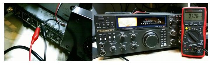
The same test is shown below but using R174 with my rig set at 14.200 MHz. I've connected a scope probe here, but a J-hook works too. To use the resistor, you will have to scrape some paint from the wire lead shown above (arrow). I would use an Exacto knife and work slowly, carefully shaving along the axis of the wire.
