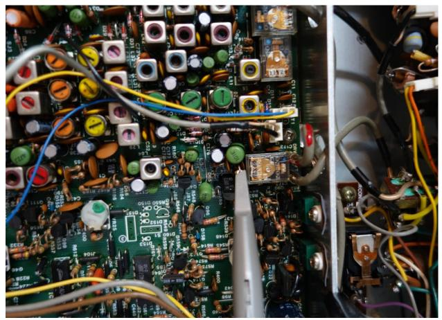
Note that I already have a probe attached to a major SU test point, R174, located just behind the transmit relay.
