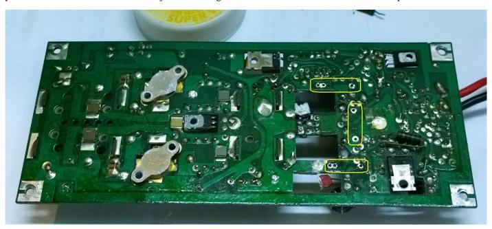
The photo below shows the finished PA board, with the new resistors outlined in red.
