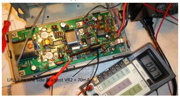
Note how Marcel lifted the side of L7 near the regulator to set the idle current. Extreme care needs to be taken here not to short anything out.. The main idle current measurement shown below is much easier.
