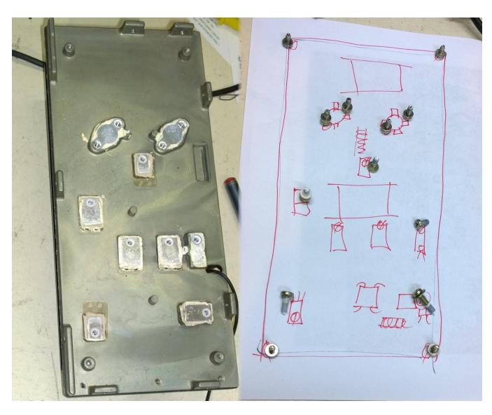
The "X's" below mark the insulator locations. The output "pills" mount right to the heat sink.
