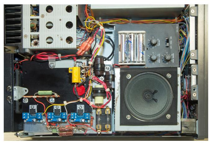
The green resistor near the top cover mounting hole is the 33 ohm feed resistor to the digital board.
