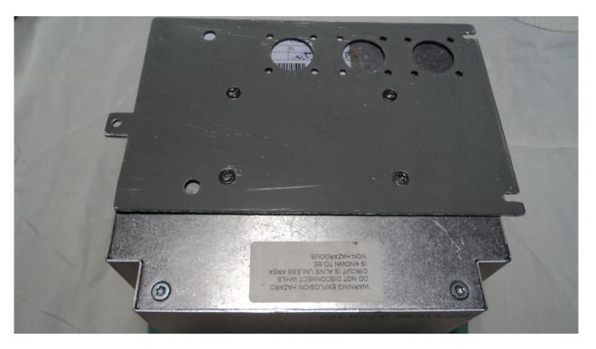
The original case-mounting bracket on the left-rear of the chassis has to be modified slightly so as to clear two of the Quint case screws. See Photo 2.
