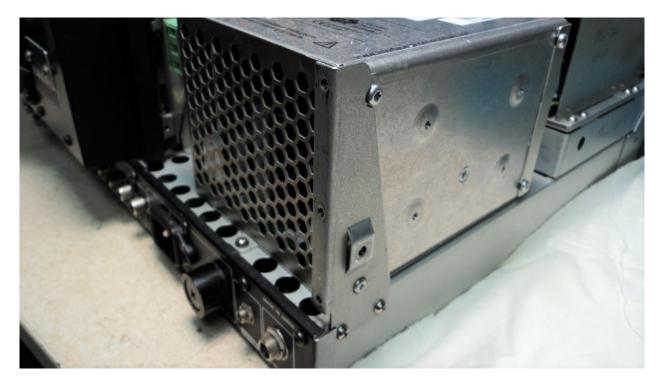
Re-use the upper case-half mounting bracket originally attached to the PS heat-sink by flattening it and pop-riveting it to the top of the fan case. See Photo 3.
