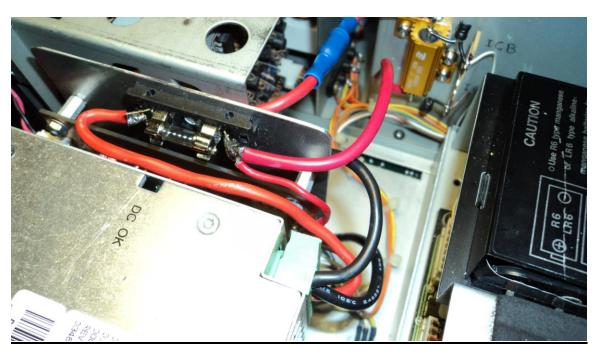
The collector current for the finals is measured using a  $.05\Omega$ , 25 Watt, metal-clad resistor and 150  $\mu$ H filter chokes soldered to a terminal strip and mounted to the wall of the Antenna Tuner unit using self-tapping screws. See photo 6. The ATU must be removed in order to drill the mounting holes. Cut off the ends of the self-tapping screws inside the ATU case or they will get *very* close to the variable capacitors.
