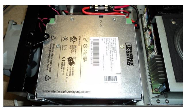
I decided to let the two fans run continuously, but changed them to a pair of very quiet NOCTUA NF-R8 redux-1200 units (available from Amazon). The PA fan blows cool air inward and the power supply fan draws warm air outward. Each is in series with an  $82\Omega$  resistor to the +15V source. See Photo 4.
