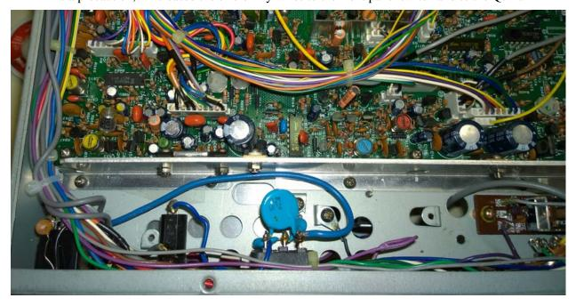
When the top cover is installed, it will press down slightly on the Quint. This isn't a problem, but it does make it nearly impossible to install a screw or something here to make the rig look stock again. I might experiment with a blind nut and a very short screw here. I would advise against drilling holes in the Quint though. If you're modernizing your power supply section, then you're probably more concerned with functionality than aesthetics anyway.
