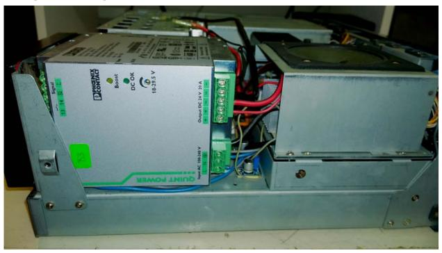
Note from the photo here that once the bottom half of the case is installed, you can still access the DC power terminals and the voltage adjustment screw. This really comes in handy sometimes.
