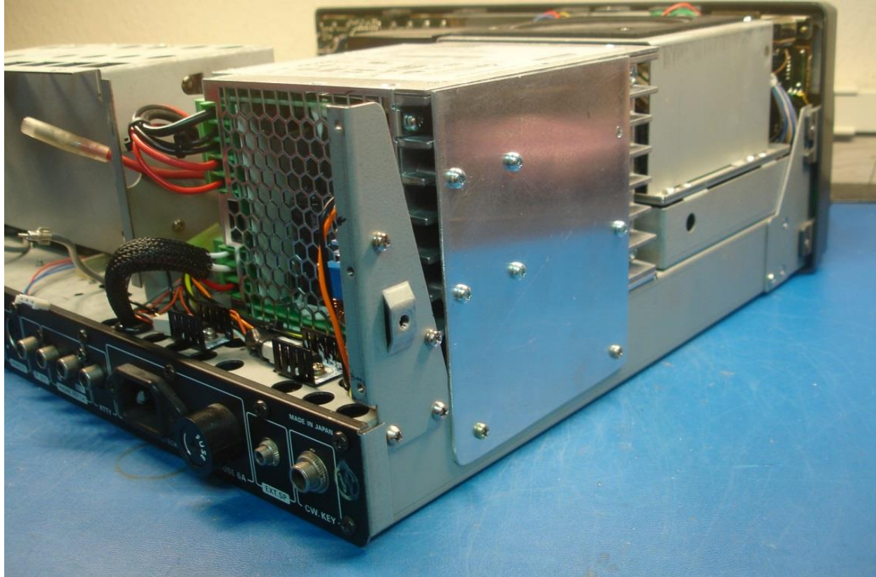
Figure 10 TS-930 UPGRADE QUINT Power Supply Mounting
