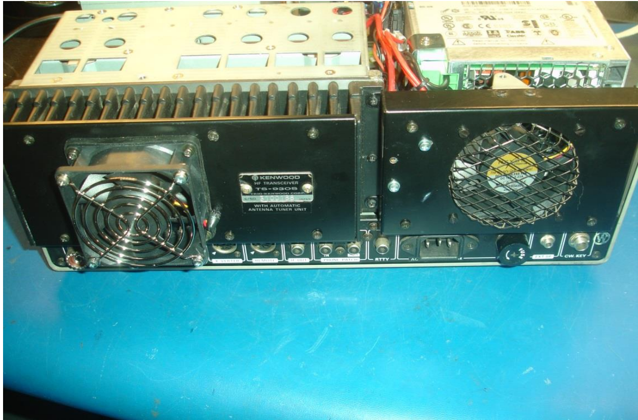
Figure 12 TS-930 UPGRADE PA Fan Replacement
