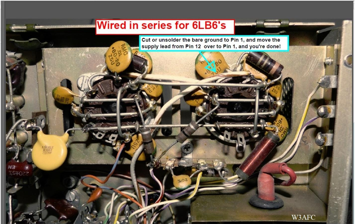
The two tubes are almost identical electrically. The 8950 has pin 6 tied to pin 2 internally, and in the rig, and the 6LB6 does not. But in this application, that doesn't make a difference.
