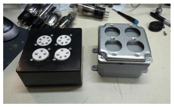
Once I decided that the outlets would fit in the smaller Carlon box, I ran with that design. This is a MUCH thicker and sturdier box, but once again I recommend cutting the socket holes by running the boring bit in reverse.
