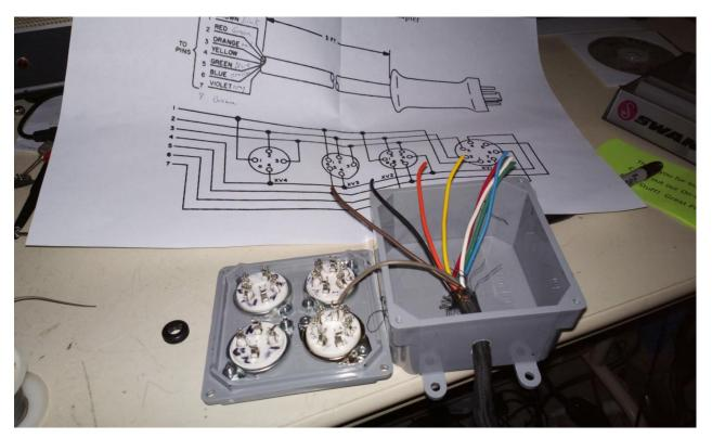
My EICO cable had eight wires for the plug, plus a floating white wire for a plate cap lead, so I had two spares that I didn't use. I considered having a plate/grid cap lead on my adapter, but the 667 has such a long built-in lead that it reaches the adapter, whether you put it in the lid, or next to it.
