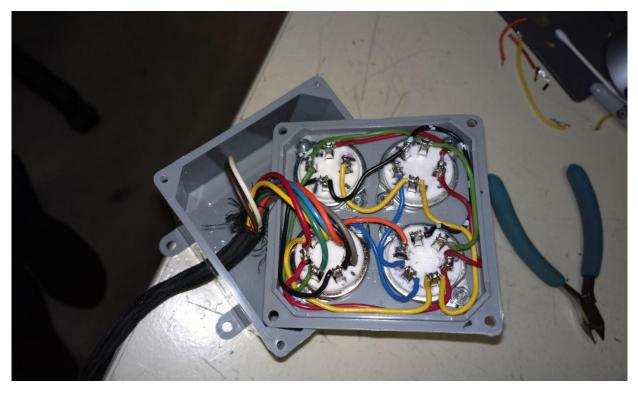
I ran all wires to the 7-pin socket first. That makes the rest of the wiring easier. Basic 18-20 gauge hookup wire works well for connecting the rest of the sockets, or you could strip some individual conductors from your 7-conductor main cable (especially if you had to buy 20 or 30 feet of it).
