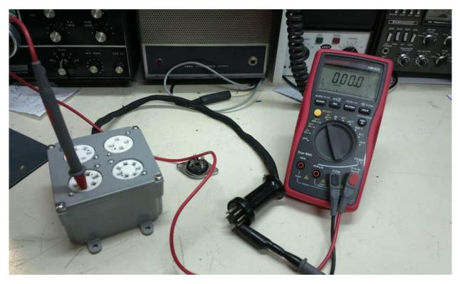
**This is a critical step**, because a wiring fault could cause damage the tube or worse, your tube tester. Once you verify that all the sockets are wired correctly, it's time to test some old tubes. This UY224 tests as a 24A. One advantage to the Carlon box is that it's cheap and it goes well with the color of the 667's case.
