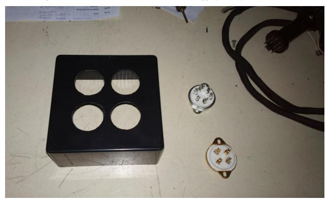
The removable top plate was very thin, so I cut my socket holes in the lower half of the box, which makes wiring the sockets difficult.
