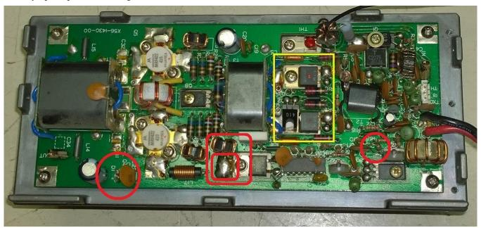
The famous "Red Dot" Motorola MRF485 driver transistors that you've probably heard about are boxed in yellow. The red dot denotes low current gain, also known as Beta or hFe. These have not been manufactured for years, as they were a special "run" for these radios by Motorola. I'll explain the red circles and squares on the following pages.
