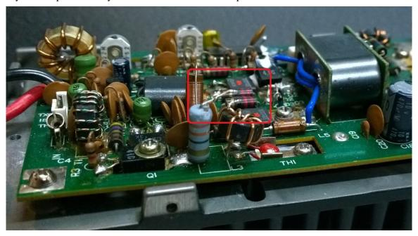
Now repeat 4a and 4b. If Q1 tests good, the problem must be either in the Final Output stage (Q4 & Q5), or the CONTROL circuitry. Reconnect L3 before putting your PA back in service.
