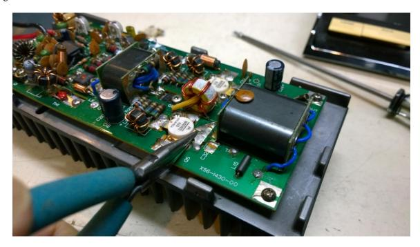
If lifting the Collector tabs causes the readings across the PA power leads to return to normal, then one or both of the Finals are leaky or shorted. If only one IS bad and you have a spare with the same color dot, then you might be able to replace just the bad final. I would use a transistor analyzer like a Peak DCA55 to make sure their gains are close. If they aren't, replace both as a pair.
