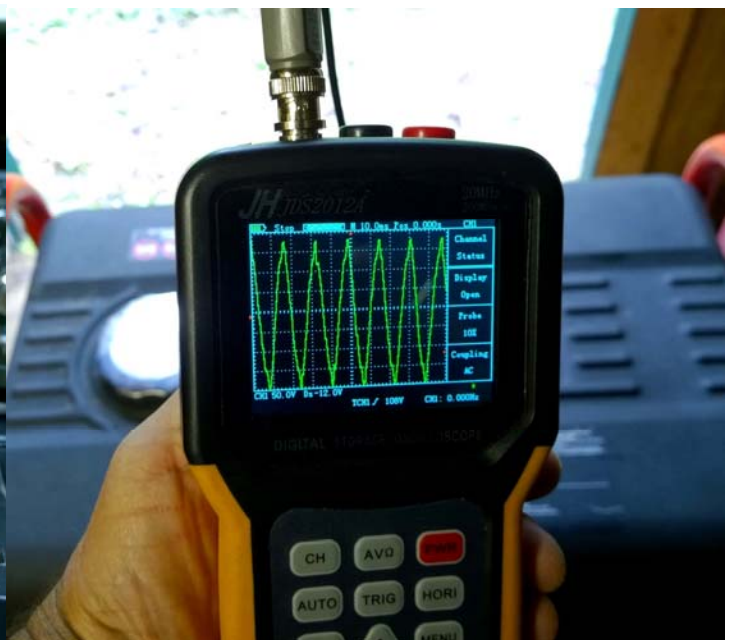
Output waveform from my Homelite generator
