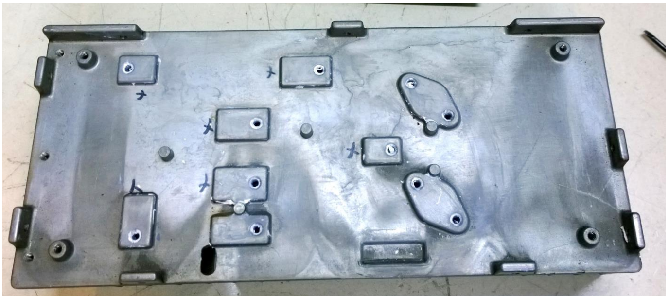
The "X's" below mark the insulator locations. The output "pills" mount right to the heat sink.
