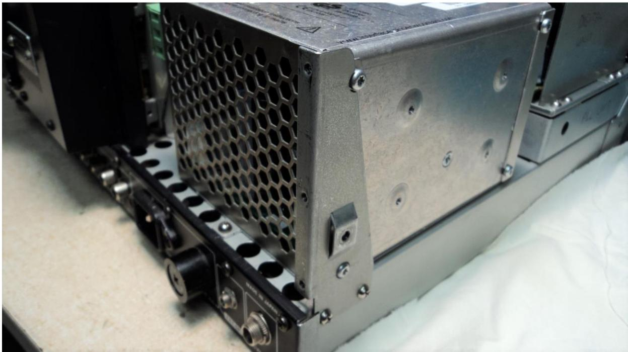
Re-use the upper case-half mounting bracket originally attached to the PS heat-sink by flattening it and pop-riveting it to the top of the fan case. See Photo 3.
