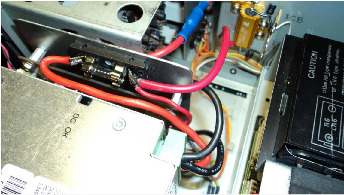
The collector current for the finals is measured using a .05 $\Omega$ , 25 Watt, metal-clad resistor and 150  $\mu$ H filter chokes soldered to a terminal strip and mounted to the wall of the Antenna Tuner unit using self-tapping screws. See photo 6. The ATU must be removed in order to drill the mounting holes. Cut off the ends of the self-tapping screws inside the ATU case or they will get *very* close to the variable capacitors.
