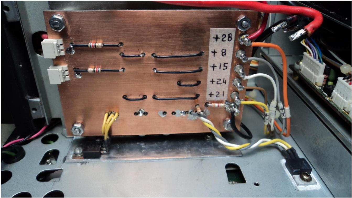
This board is mounted on stand-offs to a bent-aluminum bracket. The bracket attaches to the chassis using the old AVR board bracket mounting holes. The fan wires plug in to mating headers on the circuit board.
