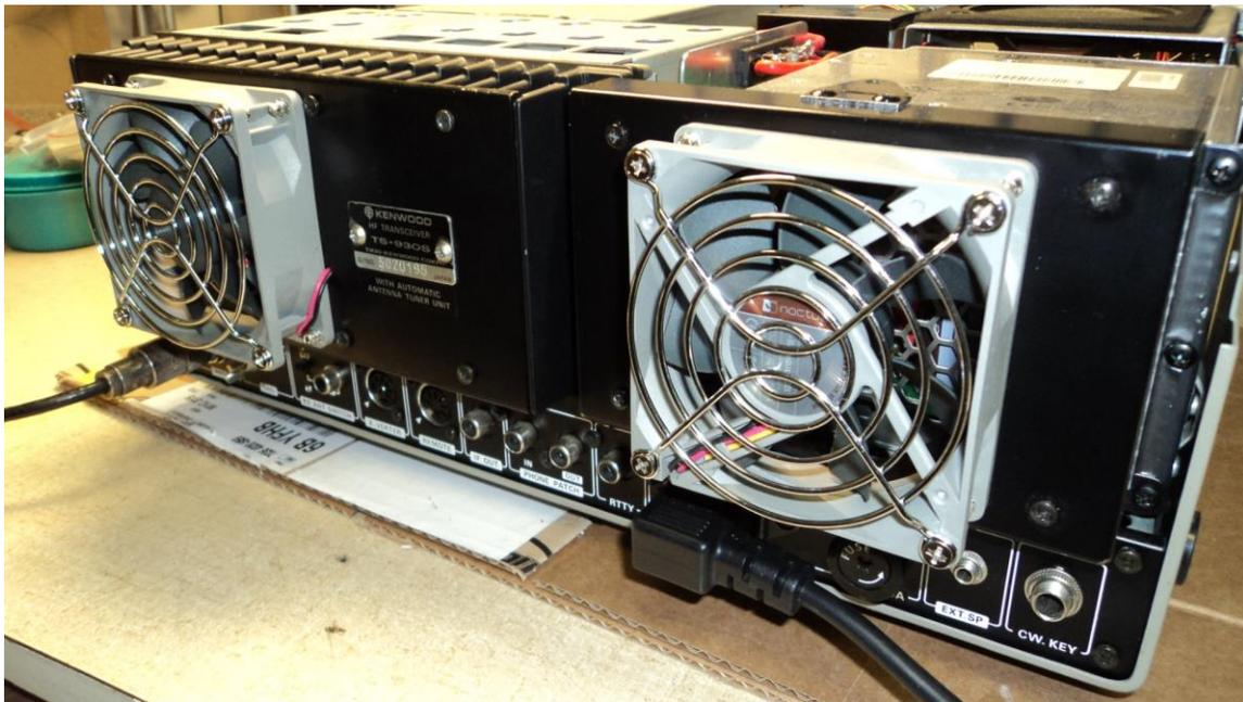
I had already done the 'W6NL mods' ( [www.kkn.net/~k5tr/ts930fix/w6nl930.pdf](http://www.kkn.net/~k5tr/ts930fix/w6nl930.pdf) ) which, amongst other things, replace the mess of under-rated resistors and Zener diodes in the power-supply fan case with 7815 and 7808 three terminal regulators bolted to the original power supply heat-sink.
