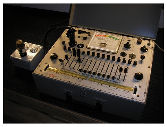
Note that I used the Chinese made ceramic tube sockets readily available as I didn't want to use any of the NOS Amphenol I77-MIP Bakelite tube sockets that I have as they are getting scarce and are very expensive when you find them. Also, I used a Heyco # 3461 cord grip for attaching the EICO CRA TV adapter cable to the box, which can be bought at a hardware store.
