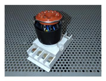
EICO 666/667: Using the 11-pin to 8-pin octal adapter shown above and a new Eimac 8122, my recently refurbished EICO 667 showed a reading of about 100, using the settings for a 6LW6/36LW6 tube and a filament voltage of 12.6 volts. The other 8122's that came in my Hurricane tested proportionally lower. They are RCA tubes, marked 3-10-2016. The best one came in at about 90, while the one with the lowest output was in the ? range, about 80.
