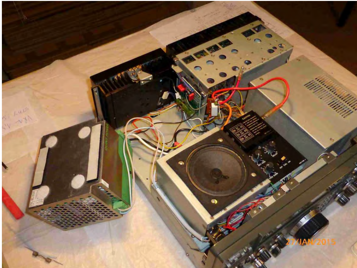
Above photo by Marcel, ON7DY. He later removed the old heat sink to improve air flow.
